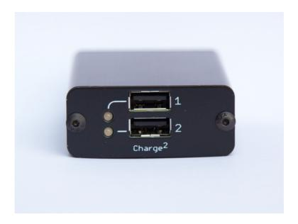
Charge<sup>2</sup> is a microcontroller controlled universal USB charger that supports the BC 1.2 specification, Chinese telecommunications standard YD/T 1591-2009, and can emulate a number of manufacturer specific chargers.
